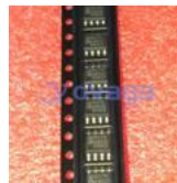
AD8170AR Analog Devices, Inc SOP8
